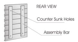
Signs provided with assembly bars must be fixed at this point. Do not fasten signs in between assembly bars unless appropriate spacers are used.
