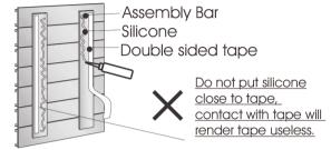
REAR VIEW - With Assembly Bars. (Signs from 147mm & up in height)
