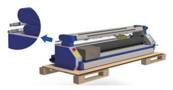
4 Lift the main part of the machine on the legs, pay attention to the alignment hole.
