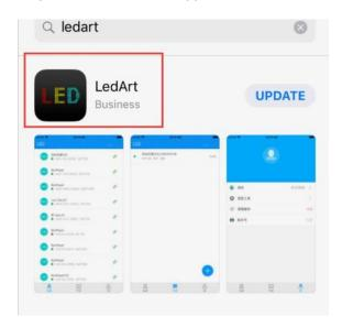
Step2: after finish installation, firstly turn the led board on, then go to "setting -> wifi" in iPhone, turn on the wifi and find the wifi network named like "D10-17-BEBB8A" or "W61-14455776637", choose it. **Notice**: the default password for wifi connection is 88888888
