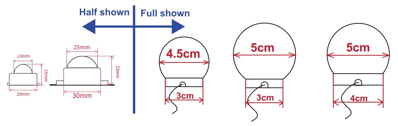
Recommended stroke needs to be 10mm larger than bulb size
