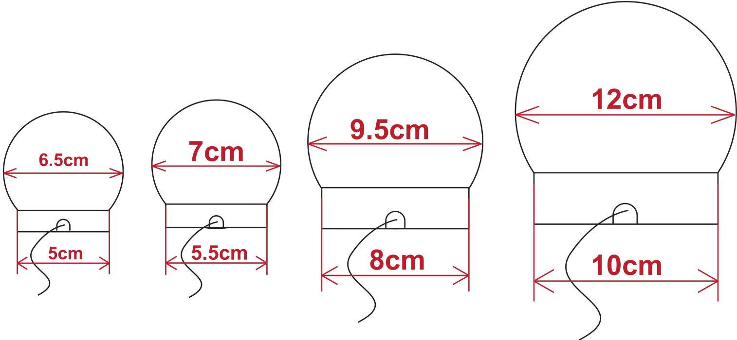
Recommended stroke needs to be 10mm larger than bulb size
